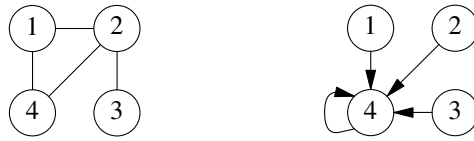
Fig. 2. A simple interference graph G (shown on the left) and its G_R (shown on the right) where R_i = 4 for each i
